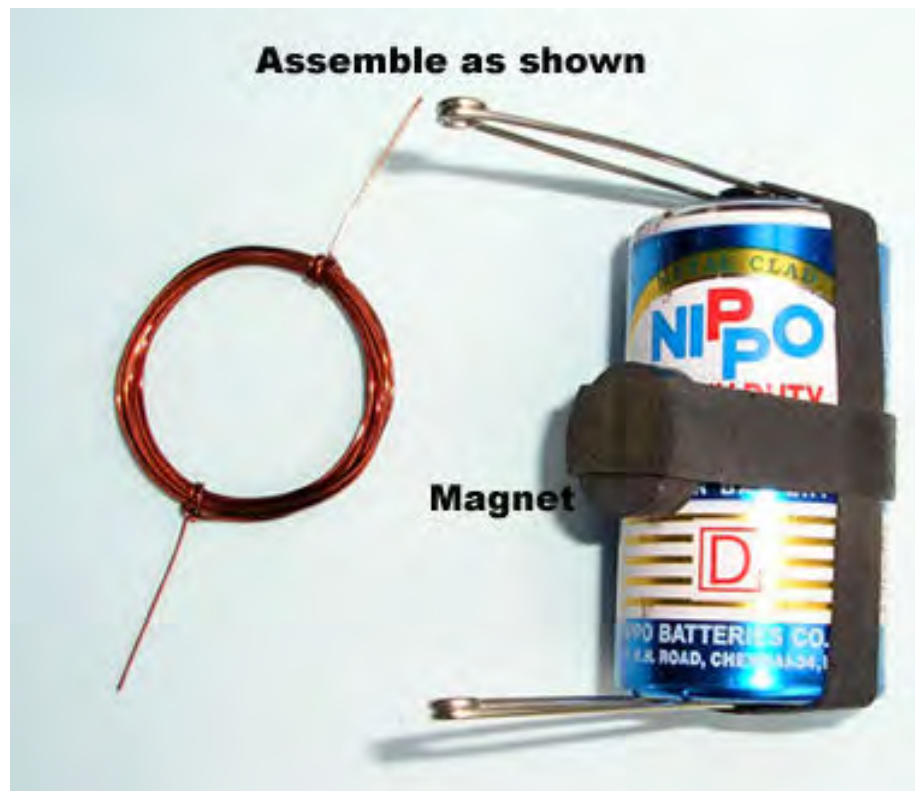
Fig. 13: Assembly of a motor. If a battery cell has a metal case, the rubber band for keeping magnet in place will not be necessary.
