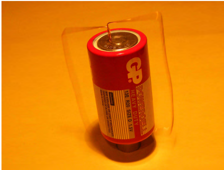
Fig. 9: A photo of a rotating motor with a frame
