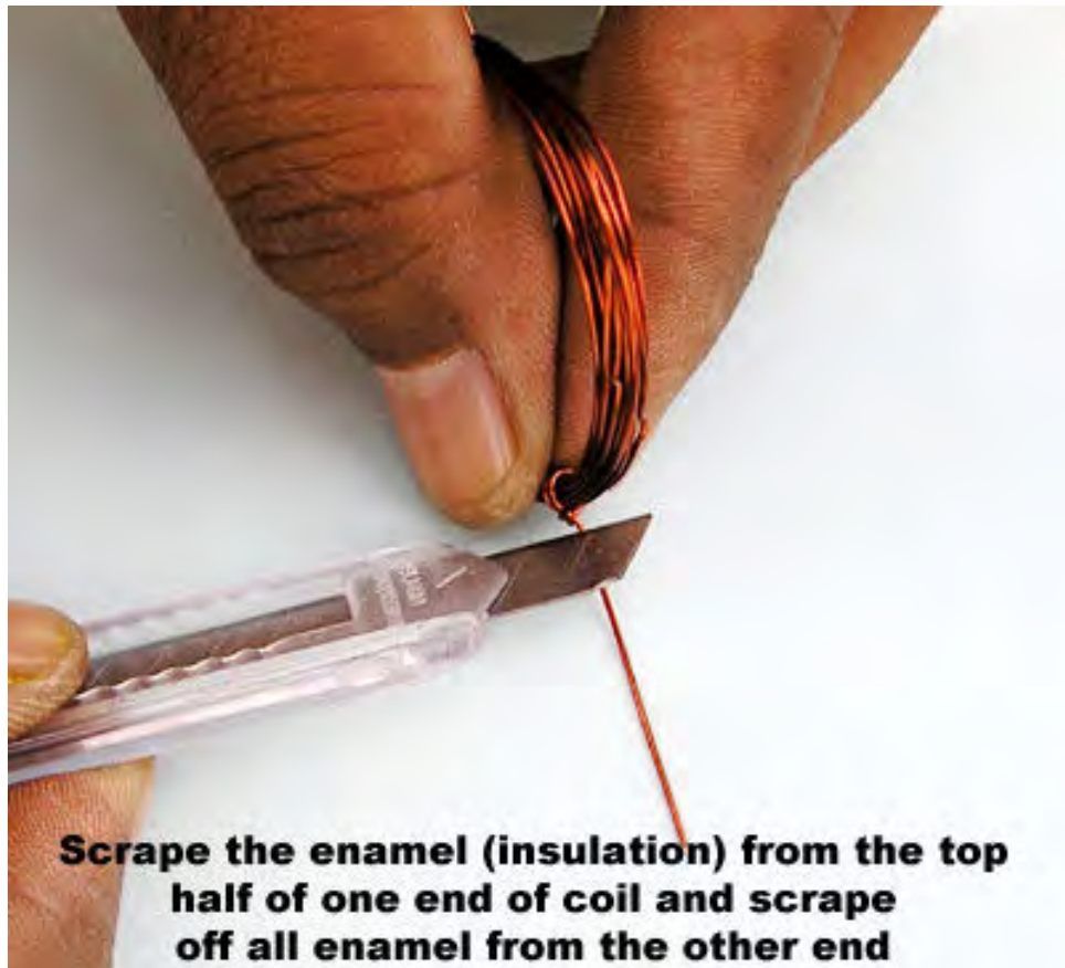
Fig. 12: Removing insulation.
